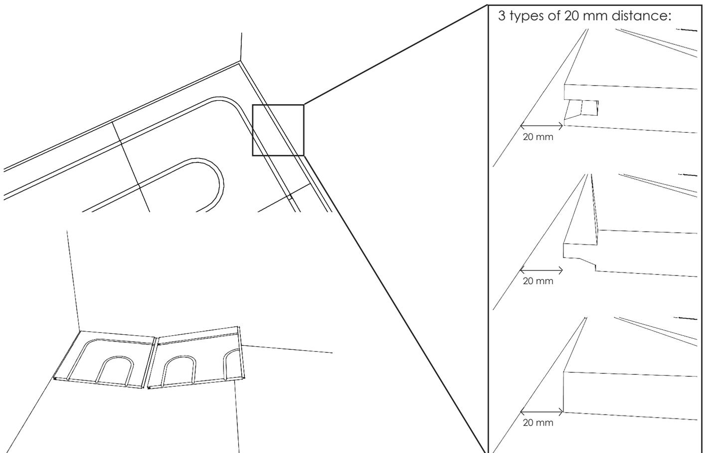
\* First 3 to 5 boards install without fixing them with screws. This gives opportunity to align the floor boards along the wall with 20 mm distance. When aligning is finished fix boards with screws (approx. 12 - 15 screws per m<sup>2</sup>).
